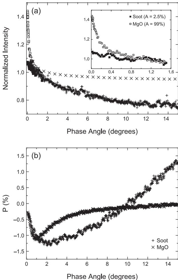
**Fig. 4.** (a) Photometric and (b) polarimetric phase curves for MgO measured with the laser laboratory photometer (open and filled squares) and the lamp photopolarimeter (crosses and pluses). The inset in the upper corner of (a) shows the small phase angle region in greater detail.
