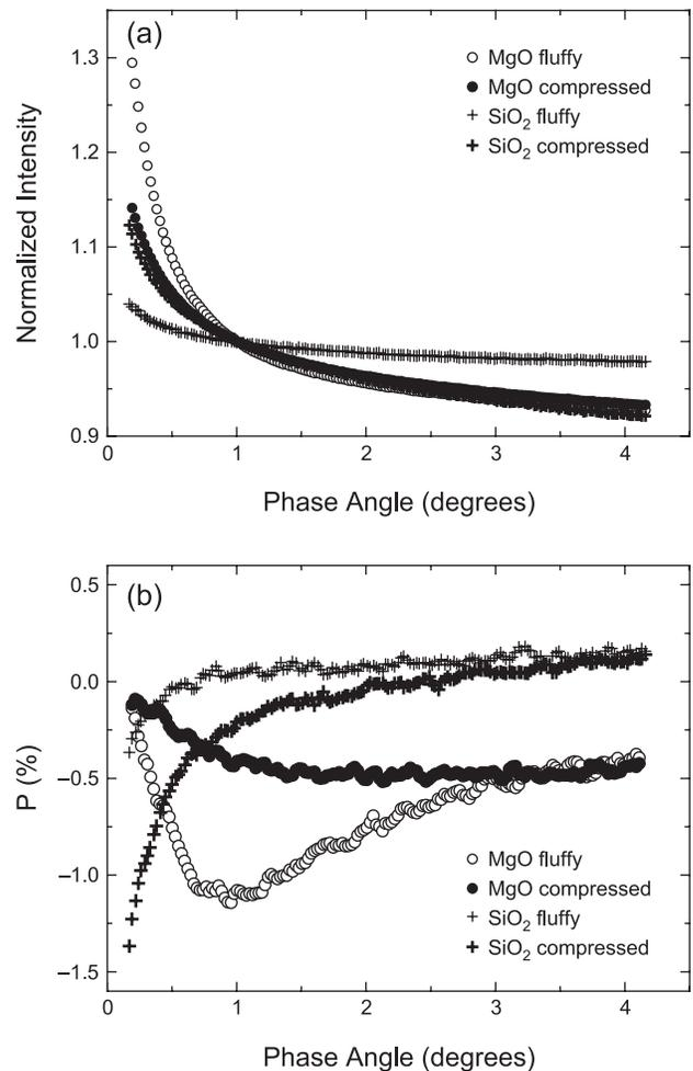
**Fig. 5.** (a) Photometric and (b) polarimetric phase curves for MgO and  $\text{SiO}_2$  before and after compressing with alcohol drying at  $\lambda = 0.63\ \mu\text{m}$  (*Shkuratov et al.*, 2002).
